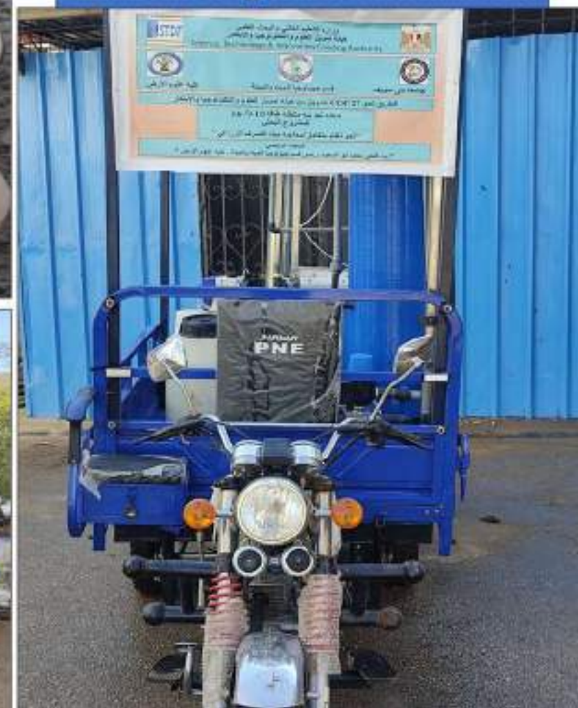
Mobile unit for agricultural wastewater reuse
