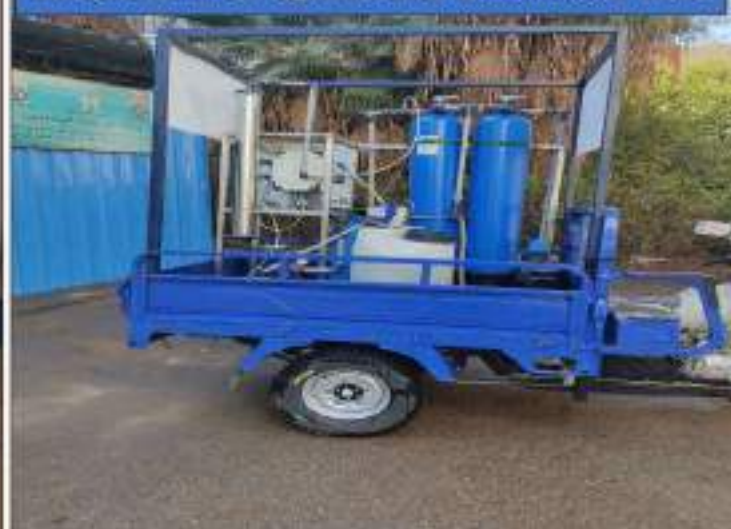
Mobile unit for agricultural wastewater reuse
